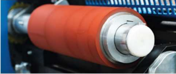
PP, Finish Folyo , Doğal Kaplama ve Laminant Malzemelerine Tutkal Uygulayan Mardane Glue Application Roller is Designed for Special Production of PP, Finish Folio, Natural Coating and Lamination
