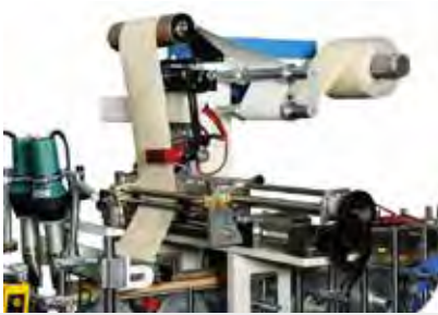
Folye Kenar Kontrol Sistemi Special Foil Edge Control System For Perfect Routing
