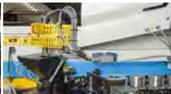
İnfraredli Ön Isıtıcı Infrared MDF pre-heater with photoelectric
